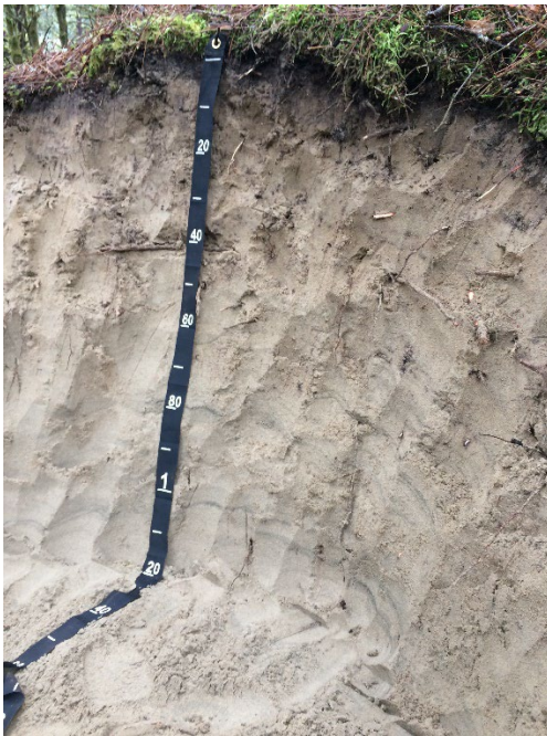
Figure 2a: Initial soil development in a coastal sand dune. Organic matter enrichment is limited to the top 10 cm (Total organic matter = 3 kg m 2 )
